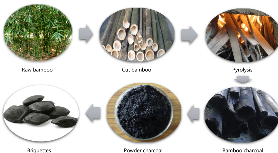
Fig 1: Schematic diagram of the bamboo carbonization process
